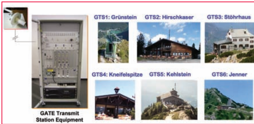
Figure 2: GATE Transmitter Locations and Transmitter Rack GATE Infrastructure Overview
